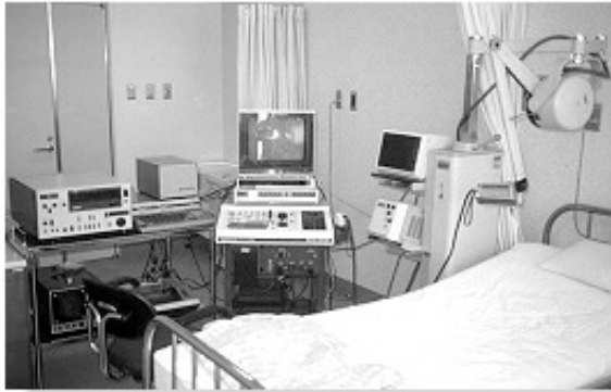
Kazunori Baba's 3-D setup in the mid 1980s. A linear array probe was mounted on an articulated arm for position sensing. On the right is the computer setup for making the calculations. (click on the picture for larger view and description)
