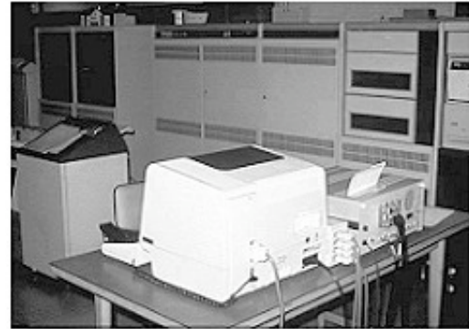
Kazunori Baba's 3-D setup in the mid 1980s. A linear array probe was mounted on an articulated arm for position sensing. On the right is the computer setup for making the calculations. (click on the picture for larger view and description)
