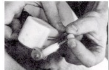
Third version of the duplex scanhead 1976. The plunger on the right moves in and out to adjust the range-gating
