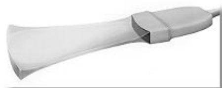
2-D arrays with focusing in two planes
